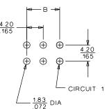
PCB LAYOUT: COMPONENT SIDE
